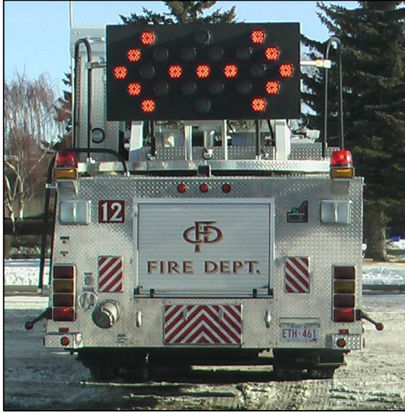
Figure 16: Calgary FD ladder truck with the arrow board on a turntable. (Courtesy of Calgary Fire Department.)
