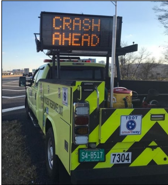
Figure 6: Sample message on a Tennessee Department of Transportation Safety Service Patrol Vehicle. (Courtesy Tennessee Department of Transportation.)
