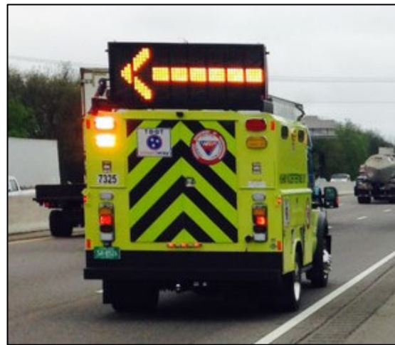
Figure 5: Rear view of a Tennessee Department of Transportation Safety Service Patrol Vehicle, with roof-mounted message board deployed. (Courtesy Tennessee Department of Transportation.)
