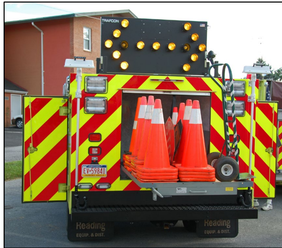
Figure 20: Gettysburg (PA) FD Fire Police unit with compartment doors open to show high visibility markings inside the doors). (Courtesy of Jack Sullivan.)
