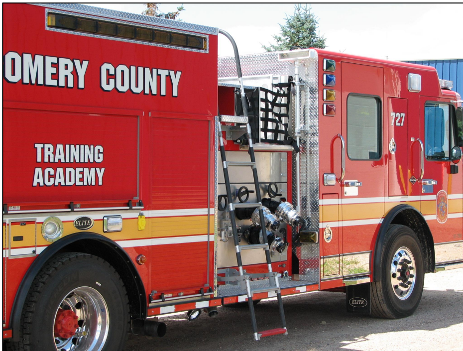
Figure 17: Montgomery County (MD) Fire Rescue engine with an arrow board on the side (top left; not illuminated). Note that the engine also has DOT reflective tape on the rub rail. (Courtesy of Montgomery County Fire Rescue Service.)
