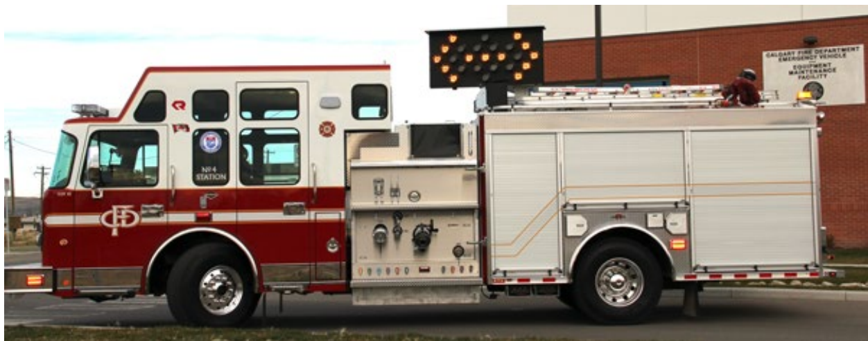
Figure 15: Calgary FD pumper outfitted with a Command Light Arrow Board that can rotate to aim at approaching traffic when parked at an angle. (Courtesy of Command Light.)
