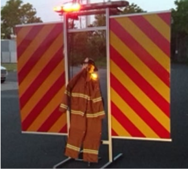
Figure 6. Photograph of the simulated firefighter with the shoulder-worn yellow flashing LED light on.
