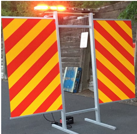
Figure 2. Photograph of the test frame with the red and yellow, full pattern of retroreflective markings.
