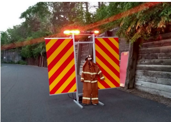
Figure 5. Photograph of the simulated firefighter located between the two panels containing retroreflective material.
